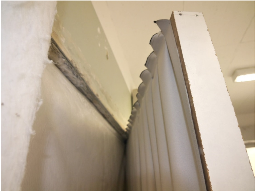
Figure B.3. Exemplary picture of a setup with one layer of molton/film in the window test stand (test setup opened).
