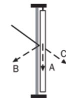
The glare protection product takes up part of the light by absorption (A), while the remaining light is reflected (B). Transmission (C) is used to describe the part of the light that can penetrate through the hanging. The glare protection product allows sufficient daylight into the room while retaining the potential for visual connection with the outside world.
