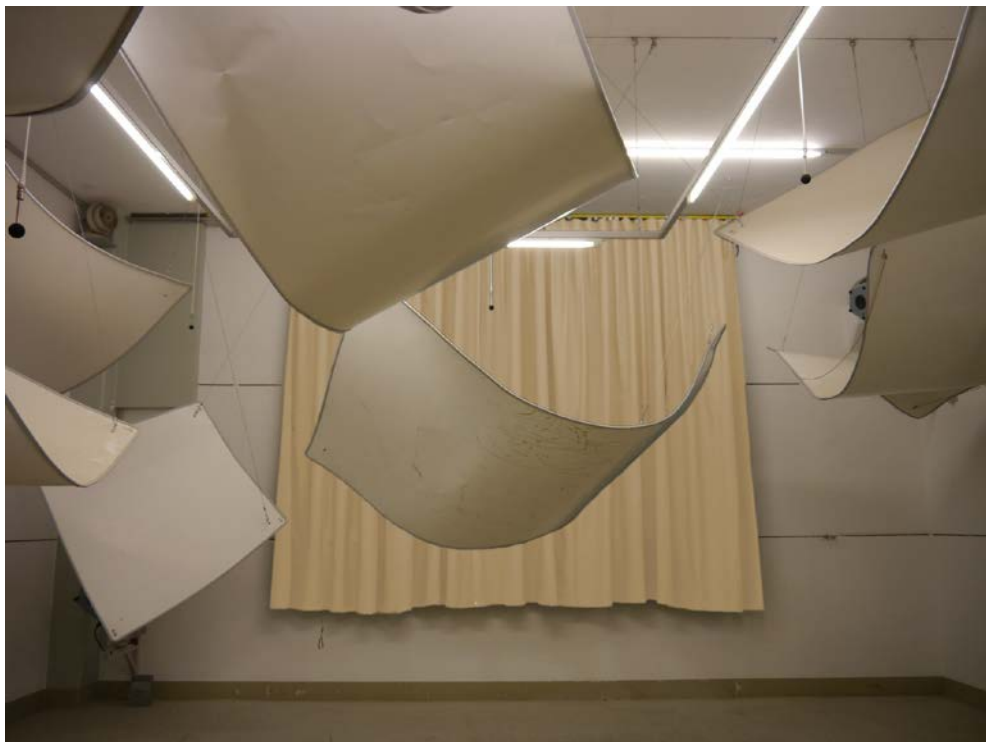
Figure B2. Folded arrangement: test object mounted in the reverberation room.
