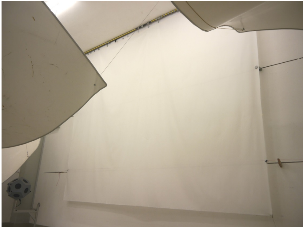
Figure B.1. Flat arrangement of the test object in the reverberation room.
